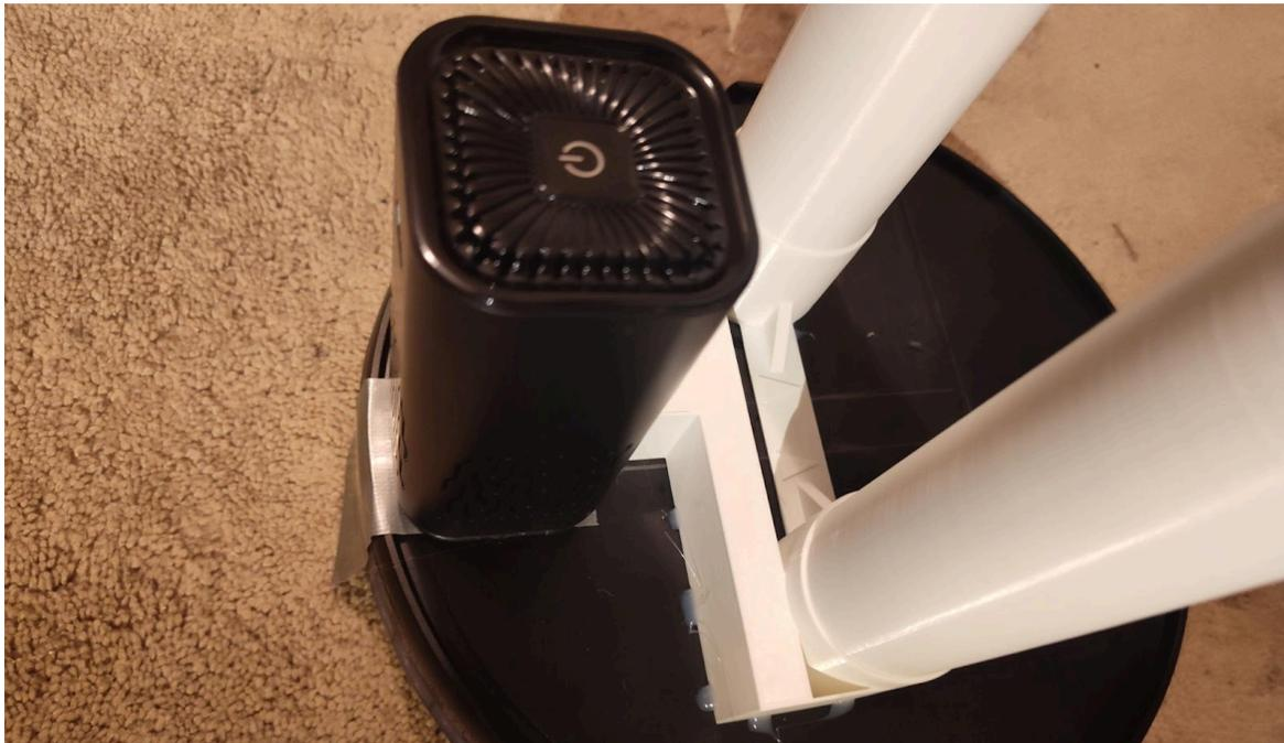
Then, put a strip of duct tape with a folded bit on the end for a tab. This will make sure the lid stays shut. Then put the air purifier (or another counterweight) on the back right against the base with a couple drops of hot glue. Make sure the plug is facing outward.
