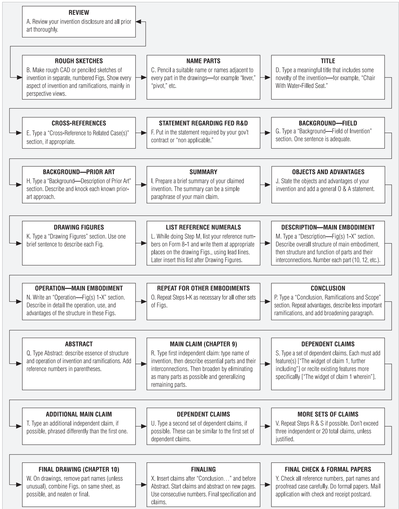
Fig. 8A—Steps in Preparing a Patent Application
