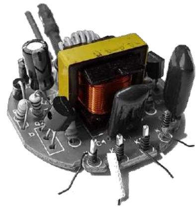
CFL power supply with desired transformer.
